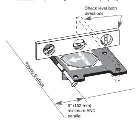
**Step 6:** Position 6" ground anchor (Item G2660) in center of hole with hinge side toward and parallel with playing surface. Using a level, ensure the anchor is level front-to-back and left-to-right. All edges of the ground anchor must be 6" (15.2 cm) away from all sides of hole and the top of the ground anchor within a range of 1"- 3" (25-75 mm) above the level of the playing surface.
