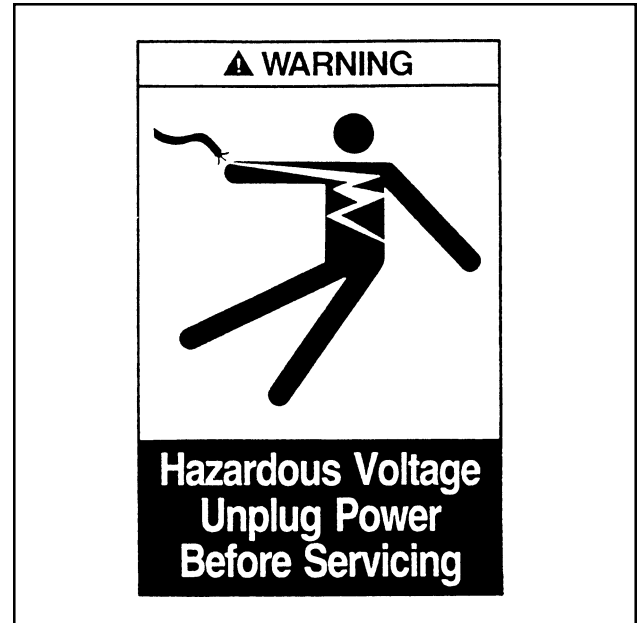
Figure 1-2 – Electrical Warning Label
