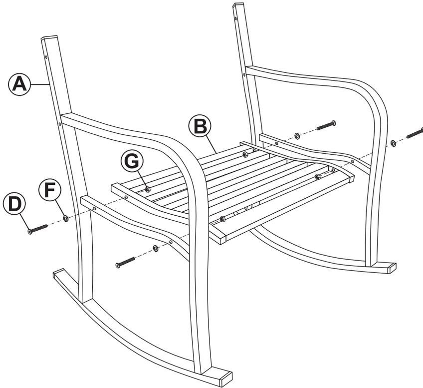
Loosely fasten two Side Panels (A) to Seat (B) by hand-tightening M6x50mm Bolts (D), Washers (F), and Nuts (G).
