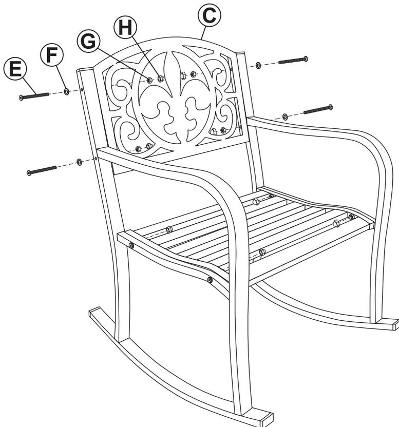
Loosely fasten Backrest (C) to the side panels by hand-tightening M6x70mm Bolts (E), Washers (F), and Nuts (G).
