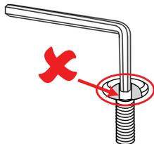
**TIP:** Always fully insert the hex key inside the designated notch on the bolt head.
