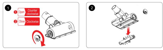
Insert a coin into the slot to disassemble the brush roll.
