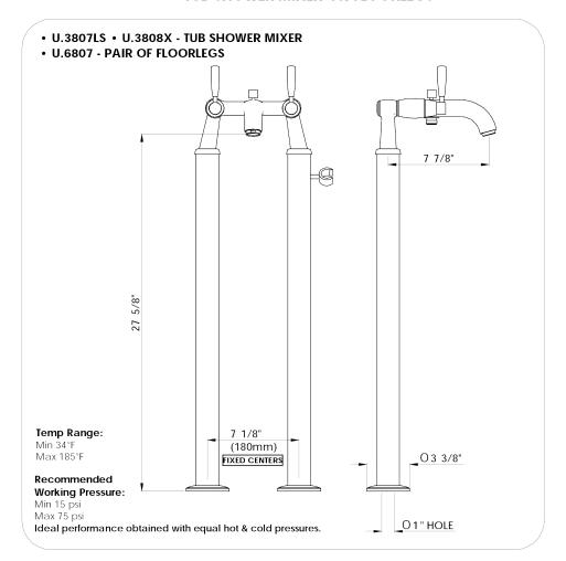
•Must be installed with a listed in-line device complying with ASSE1070
