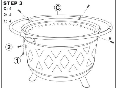
Insert one Safety Rings (C) into another and loosely secure them by hand-tighten the rings to the fire-bowl using M6x12mm Bolts (2). Then, loosely connect the remaining two rings to the fire-bowl.
