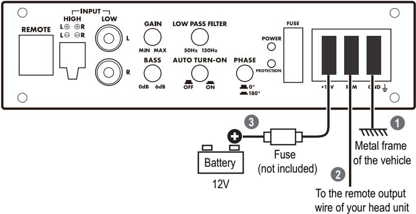
1. Using an 8 gauge (or heavier) wire, connect the **GND** terminal on the subwoofer to the metal frame of your vehicle. Keep the ground wire less than 39" (100 cm) in length.
