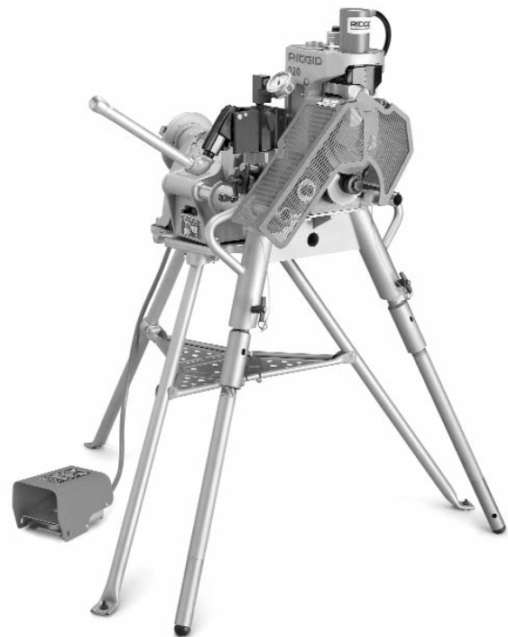
Figure 2 – 920 Roll Groover Attached to 300 Power Drive
