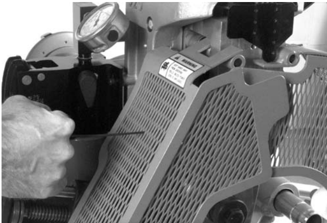
Figure 18 – Loosening Set Screw In Upper Roll Housing
