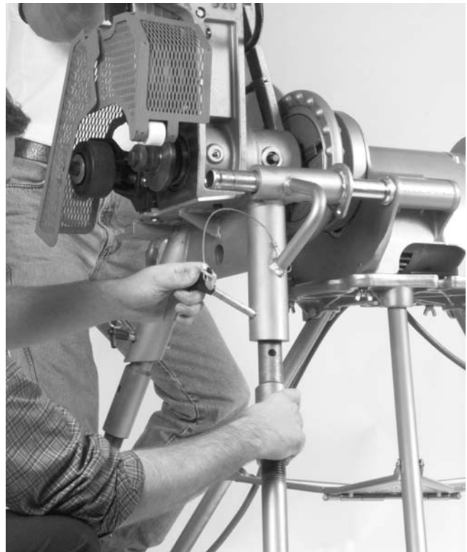
Figure 23 – Removing Legs From Base
