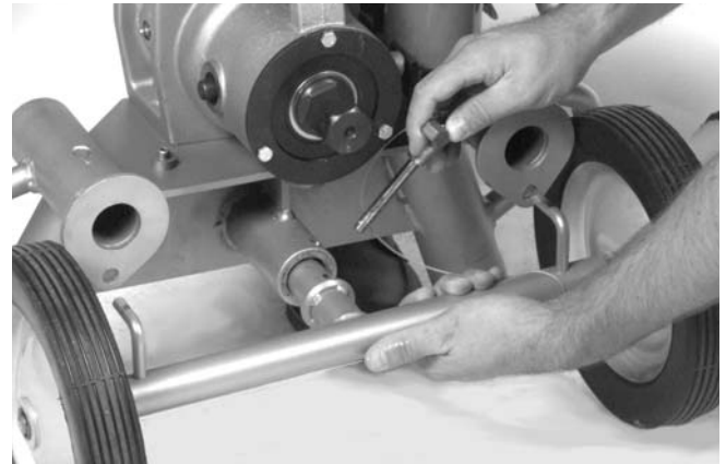
Figure 3 – Removing Transport Cart
