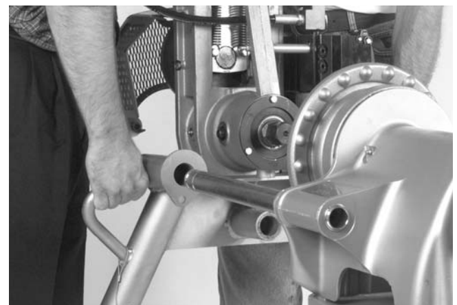
Figure 4 – Sliding Roll Groover Onto Support Arms
