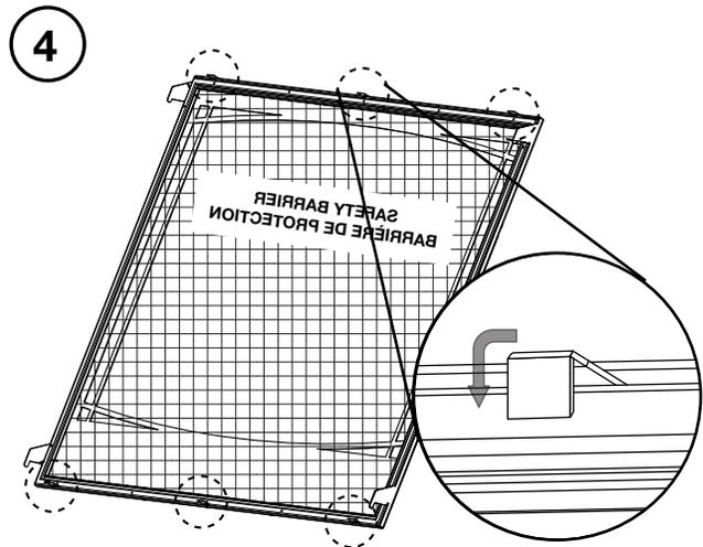
Bend 6 tabs to secure barrier in place.
