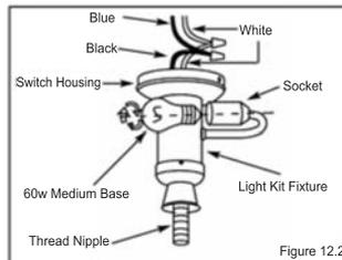
6. Carefully push all wires back into the switch housing. Then attach housing cover plate to switch housing with the 3 screws provided.
