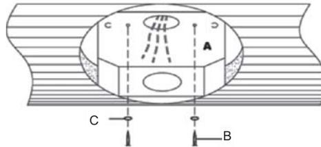
3. Attach the mounting plate(1) to the ceiling outlet box(A) with screws and washers provided with the fan , and then tighten them.
