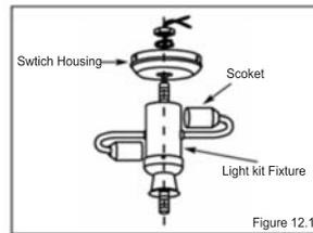
2. Locate two wires in the switch housing (white and blue labeled " for light"). Connect them to the light kit wire connectors (Fig. 12-2)
