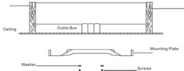
4. Insert one end of the mounting bracket through the slot on the mounting plate all the way to the end.
