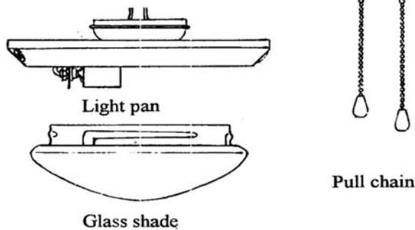
2. The whole light kit assembly includes the above parts. Locate these parts from the package and be careful not to damage the glass shade.
