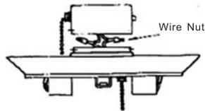
3. Carefully push all wires back into the switch housing. Then attach housing cover plate to switch housing with the 3 screws provided.
