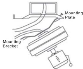
5. Hold the motor upright and adjust the motor to align the three holes on the mounting bracket with screws. Tighten the screws
