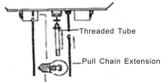
5. Attach the glass shades to the light kit, and screw up the finial. Do not over-tighten the finial , glass may break. Slide the bowl glass over the threaded nipple, followed by the cap, and then finial. Twist finial clockwise until snug (see figure)
