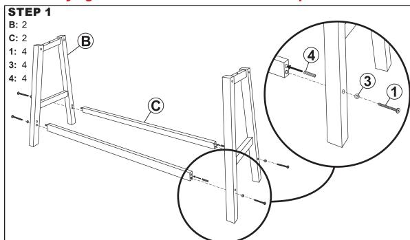
**IMPORTANT:** Do not install wood dowels into mounting holes with threaded inserts.
