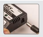
Place the charger on a flat, heat resistant surface with a good airflow all around. Connect the supplied 2S 1000mAh Li-Po battery to the charger using the white three pin balance plug, ensuring the correct orientation of the plug. The red and green 'Charger' LEDs will light indicating that the battery is charging. When fully charged the red LED will remain glowing the green will be out, whereupon the battery can be disconnected.
