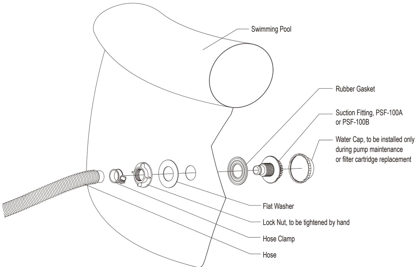
9. PSF-100A or PSF-100B Suction Outlet Fitting is to be replaced every 5 years.
