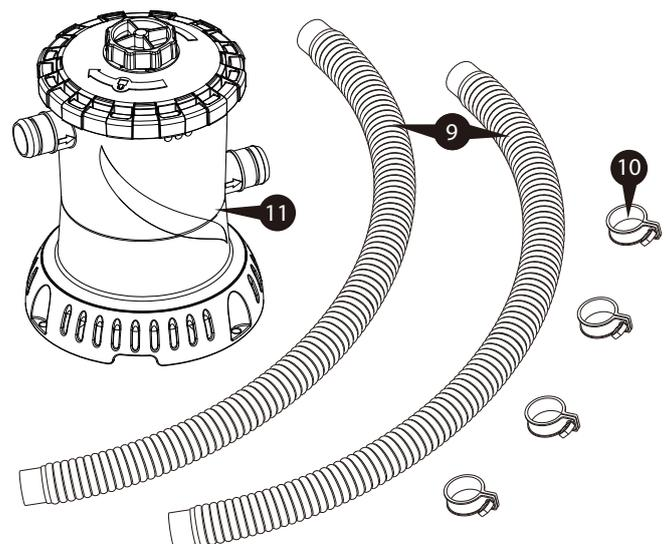
5. Connect the Suction Fitting **2** to the Pump inlet with a Hose and one Clamp on each end. Make sure the Hose Clamps **10** seals tightly over both the Hose **9** and O-Rings **27**.
