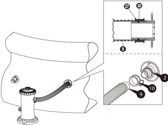
7. Tighten all the Clamps **10** to prevent water leakage.
