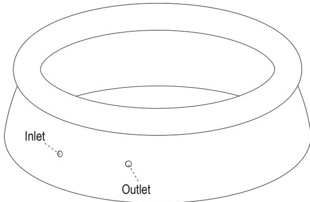
2. From inside the pool, install the Suction Fitting **2** into the Outlet opening.
