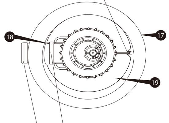
Make sure that the Rubber Nozzle **18** is aligned with the Canister outlet.
