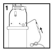
Insert the barrel connector on the CXR extension cable into the corresponding receptacle on the CXR under-counter assembly.
