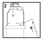
Insert the barrel connector on the power adapter into the corresponding receptacle on the CXR under-counter assembly.
