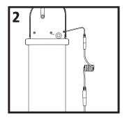
Insert the barrel connector on the power adapter into the corresponding port on the CXR extension cable.
