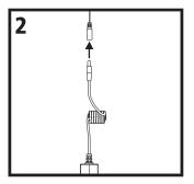
Insert the barrel connector on the power adapter into the corresponding port on the CXR splitting cable.
