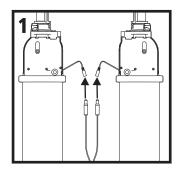
Insert the barrel connectors on the CXR splitting cable into the corresponding receptacles on the separate CXR under-counter assemblies
