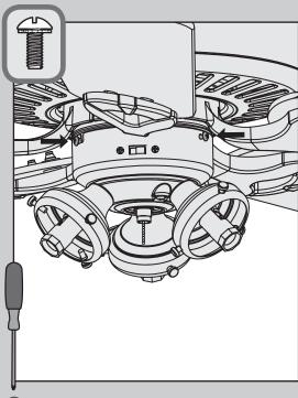
Install the third switch housing screw.
