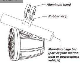
Place two supplied rubber strips around the cage bar to prevent abrasion and secure clamping. Then push two supplied aluminum bands over the cage bar, and align the aluminum bands with the metal base on the speakers.
