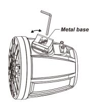
Twist the metal base to determine the optimal mounting angle for the speaker on the cage bar. Then secure the metal base by tightening the two screws.
