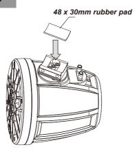
Place a supplied rubber pad (48 x 30 mm) on the metal base of the mounting band to prevent abrasion and secure clamping.
