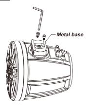
To adjust the mounting angle, loosen the metal base of the mounting band by unbolting the two screws.
