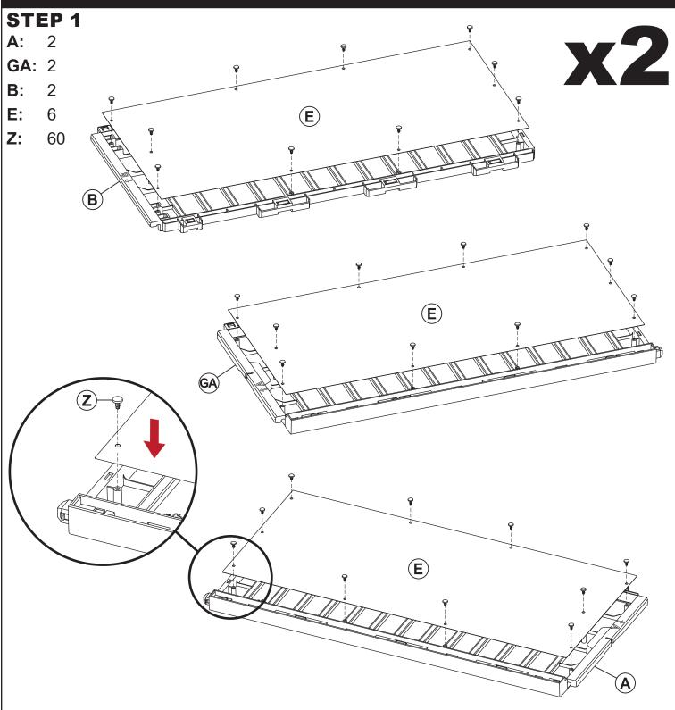
With the front sides facing down, lay out two Left Panels (A), two Right Panels (GA) and two Back Panels (B).
