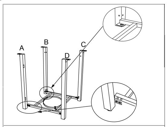
1.Connect the tank holder/base (I) With table Lets(A/B/C/D) by 6pcs screws (O).
