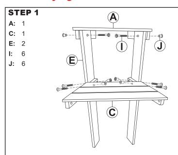
Fasten two Top Tier Legs (E) to the inside of Top Shelf (A) by hand-tightening two 35mm Bolts (I) and two Joint Connector Nuts (J).
