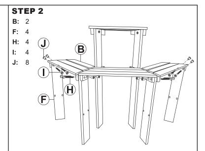
Attach Middle Tier Leg (F) to the inside of the outer edge of Side Shelf (B) using two 35mm Bolts (I) and two Joint Connector Nuts (J).
