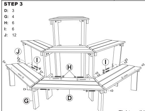
Align Bottom Tier Leg (G) with the front, left, inside edge of Bottom Shelf (D). Loosely secure by hand-tightening one 35mm Bolt (I) and one Joint Connector Nut (J).
