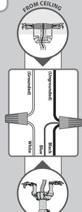
Using the orange wire connectors from the hardware bag, connect the black wire (ungrounded) from the ceiling to the black and the blue wires from the fan. Connect the white wire (grounded) from the ceiling to the white wire from the fan.
