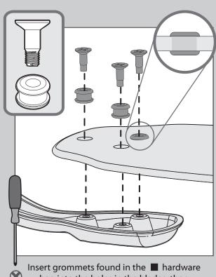
bag into the holes in the blades, then secure each blade to a blade iron with screws found in the hardware bag.
