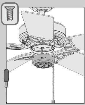
Lift the lower switch housing until its screw holes are aligned with the screw holes in the upper switch housing. Install the three switch housing screws, found in the hardware bag. Tighten all three screws.
