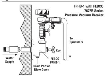
**Note:** PVB's must be installed a minimum of 12" above the highest point of water in the sprinkler system.
