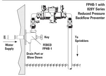
Note: RPZ's must be installed a minimum 12" above ground level.
