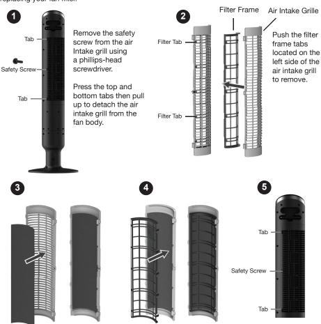
Place the filter inside of the air intake grille.
