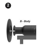
Lay product down on a flat surface. Attach base to the body, using alignment pin as a reference.
