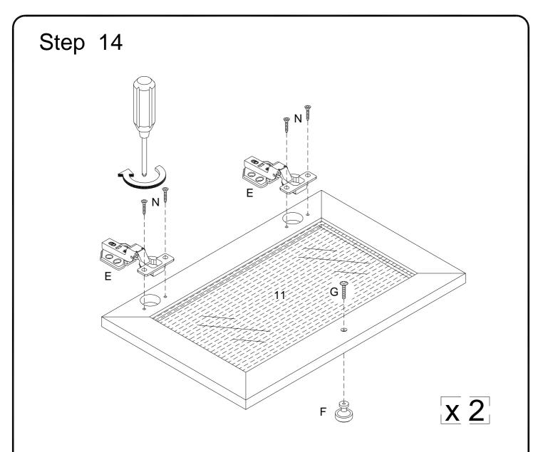
Using screw (N) attach Europe hinge (E) into part (11) , then using handle bolt (G) secure handle (F) to part (11) with Philips head screwdriver as per diagram.
