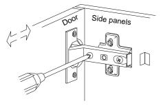
Horizontal by screw adjustment In-and-Out by loosening the hinge-arm mounting screw or via cam adjustment
