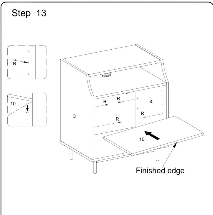
Insert shelf support pin (R) into parts (3,4) as per diagram. Make sure you place the shelf support pins (R) in the same level. So the shelf is not titled .Put part (10) into unit as per diagram. Tilt and rest the adjustable shelf (10) onto the shelf support pins .
