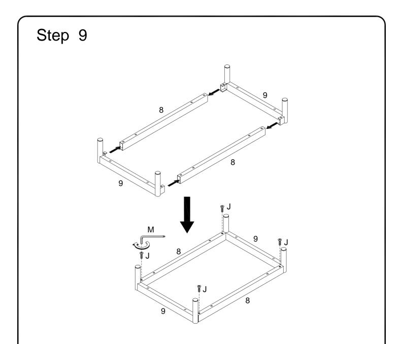
Attach parts (9) into part (8) ,then using bolt (J) secure part (8) to part (9) with hex key (M) as per diagram.
