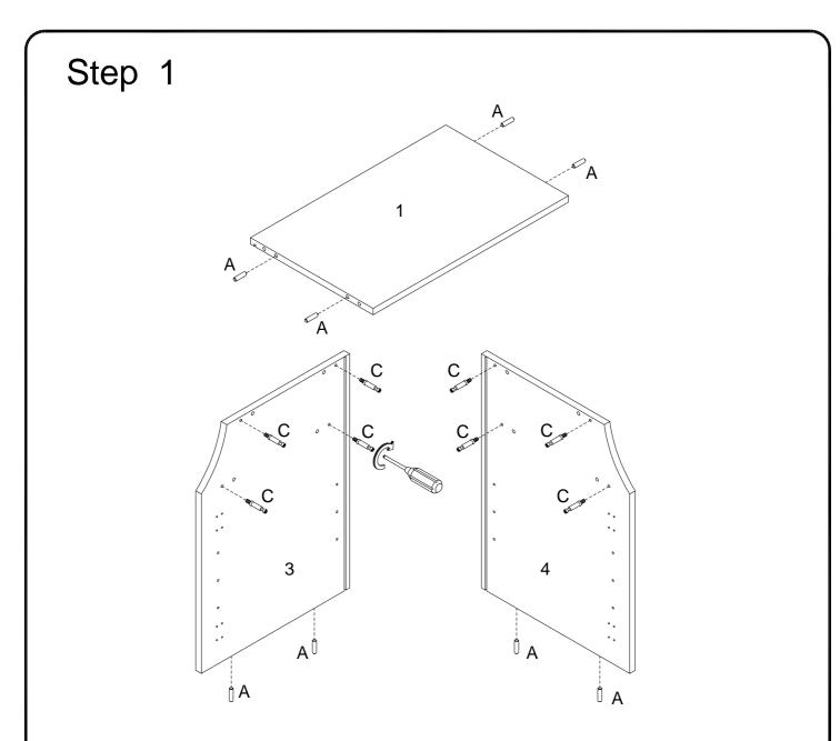
Insert wooden dowel (A) into parts (1,3,4), then secure cam bolt (C) into parts (3,4) with Philips head screwdriver as per diagram.
