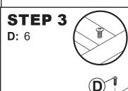
TIP: To maximize evenness, do not fully tighten a single bolt before moving onto the next. Instead, gradually tighten each bolt until all bolts are evenly secured.
