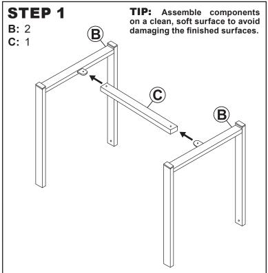
Align Crossbar (C) with the tabs on the bottom of Legs (B). Ensure the mounting holes on the crossbar are facing the bottom of the table, as shown.
