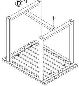
Secure the crossbar to the legs using two M8x20mm Bolts (D) and four bolts to secure the legs to the tabletop.
