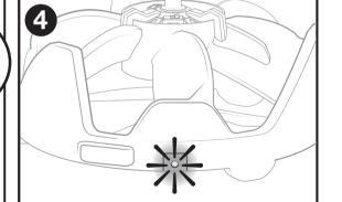
**4.** Blinking LED indicates battery is charging. Solid LED indicates the battery is fully
