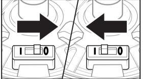
If the GRAVITOR™ has a hard crash, the motors will turn off. You will need to turn it OFF and back ON to restart it.
