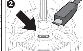
2. Plug the small end of the charging cable into
