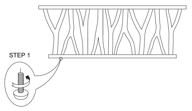
Adjust Leveler if needed to level table on uneven floor.
