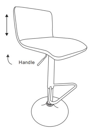
To raise the seat, lift your weight off the seat and reach underneath the right side of the Chair to lift the handle up slowly with a clockwise twisting motion to allow the Chair to rise to desired height.
