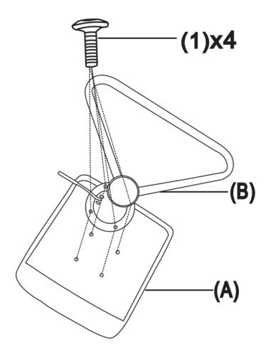
Place the Chair (A) on its back on a flat smooth surface. Attach the Footrest (B) to the bottom of the Chair (A) with four Bolts (1).
