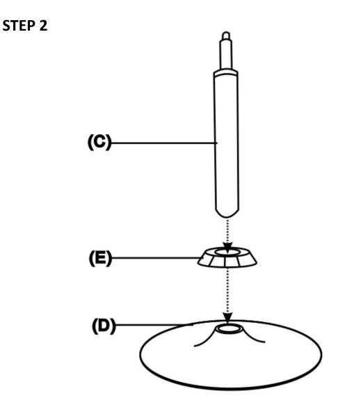
Place the Base (D) on a flat smooth surface. Attach the Plastic Ring (E) to the Base (D). Attach Gas Lift (C) to the Base (D)
