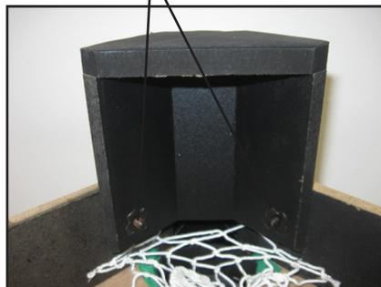
Legs to be black injection moulded ABS and should flush mount to table securely with 2 bolts, washers and nuts.
