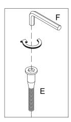
Position bottom panel (2) onto the inserted wood dowels and keep the groove have a good fit with back panel. Use bolt (E) attach part (2) into parts (3,4) with hex key (F) as per diagram.
