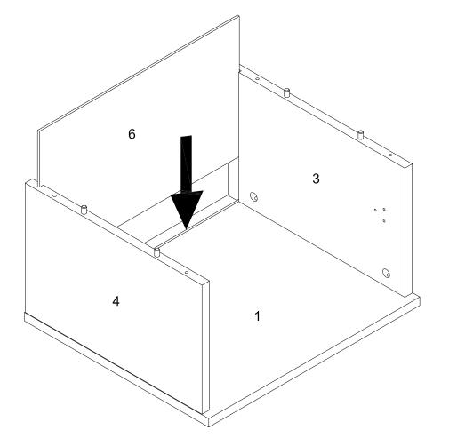
Put part (6) into parts (1,3,4) as per diagram.
