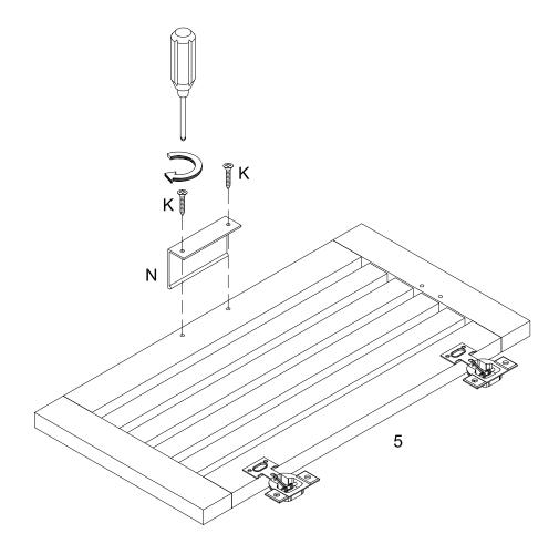
Using screw (K) attach knob (N) into part (5) with Philips head screwdriver as per diagram.
