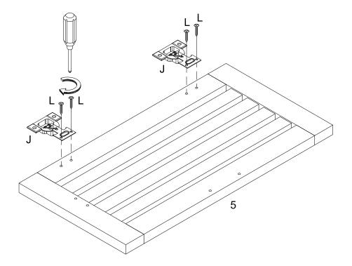
Using screw (L) attach Europe hinge (J) into part (5) with Philips head screwdriver as per diagram
