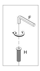
Using bolt (H) attach part (7) to part (2) with hex key (F) ,and tighten all the bolts .
