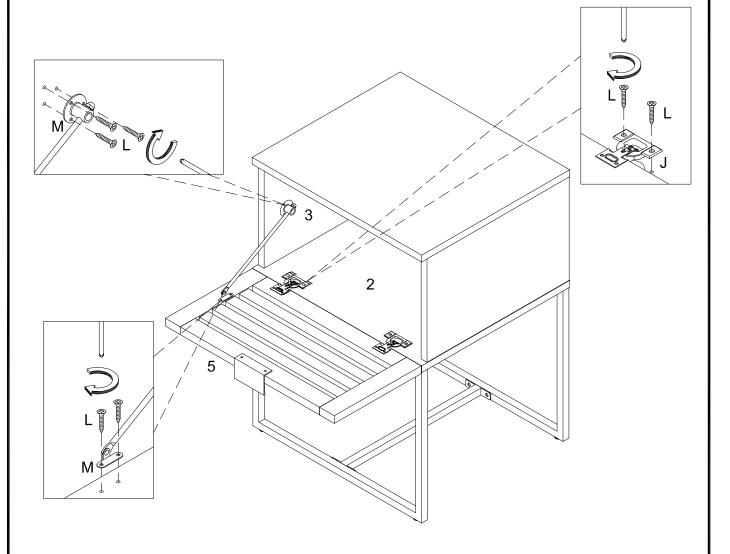
Using screw (L) attach Europe hinge (J) into part (2) ,then using screw (L) attach door hinge (M) into parts (3,5) with Philips head screwdriver as per diagram. Open and close the door to make it sure was shut correctly .If necessary ,adjust the screws for a good fit .
