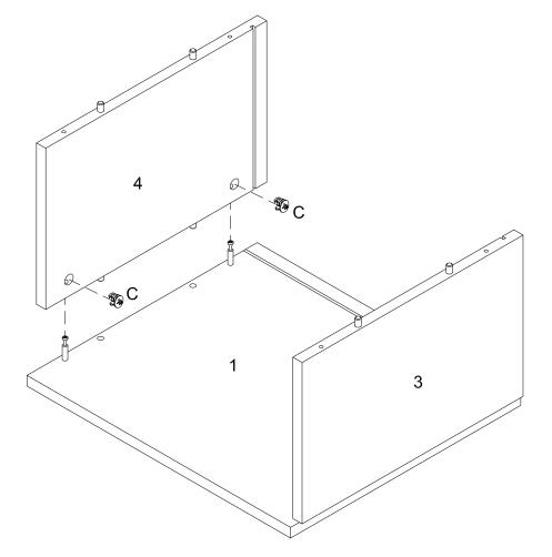
Using cam lock (C) secure part (4) to part (1) with Philips head screwdriver .
