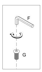
Using bolt (G) attach part (8) into part (7) with hex key (F) as per diagram.
