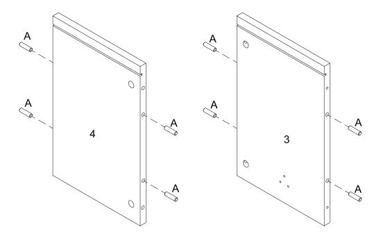
Insert wooden dowel (A) into parts (3,4) as per diagram.
