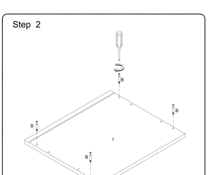
Secure cam bolt (B) to part (1) with Philips head screwdriver .
