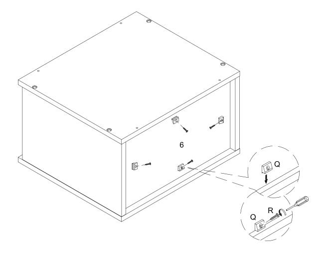
Using screw (R) secure plastic wedge (Q) to part (6)with Philips head screwdriver as per diagram.
