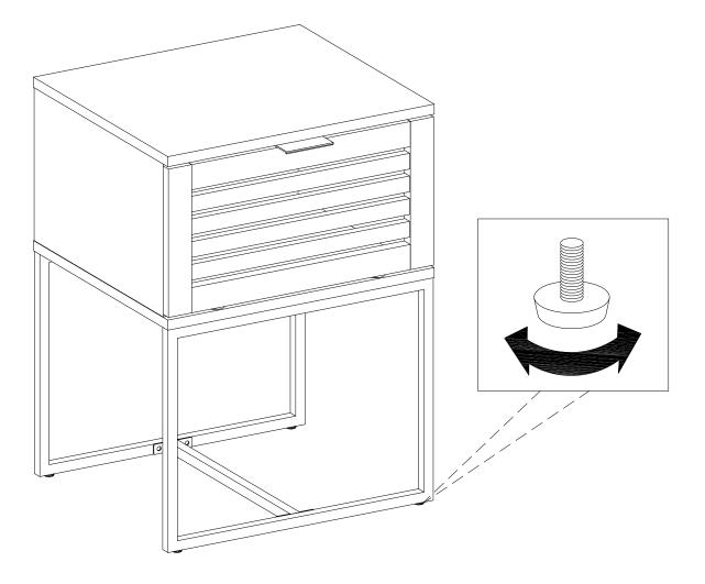
Position the assembled unit at the desired location .If necessary, adjust the floor levelers at the bottom of the legs to the level the unit .
