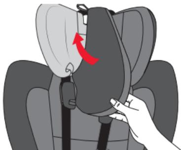
10. Replace the elastic straps and snaps at the back of the headrest.
