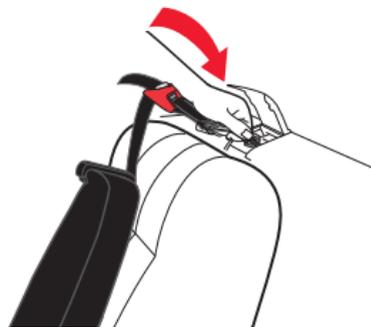
5. Squeeze handle on LockStrong belt tensioner until lock indicator turns RED, then lift up on belt tensioner to allow access to the belt path.
