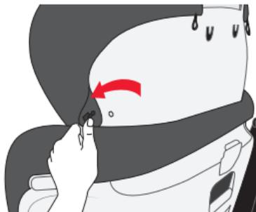
4. Pull the harness strap out of the opening in the headrest pad, and remove headrest pad from seat.
