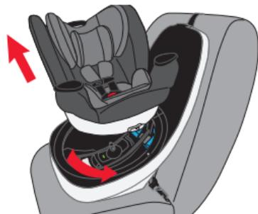
2. Disengage LATCH/UAS connectors on both sides of Car Seat (see pg. 48), then open LockStrong.
