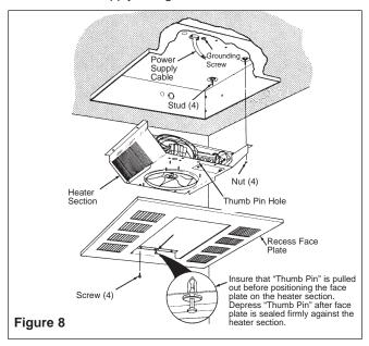
13. Push the heater section onto the studs and securely tighten four nuts (supplied) on the studs to secure the heater section to the recess mounting box (Figure 8).
