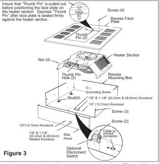
heater section to the recess mounting box (Figure 3).
