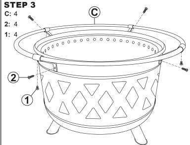
Insert one Safety Rings (C) into another and loosely secure them by hand-tighten the rings to the fire-bowl using M6x12mm Bolts (2). Then, loosely connect the remaining two rings to the fire-bowl.
