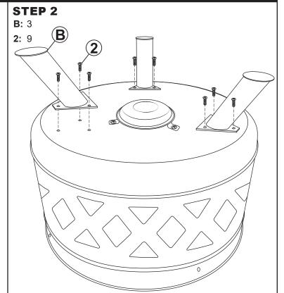
Align one Leg (B) with the bottom of the fire-bowl and securely fasten using three M6x12mm Bolts (2). Repeat to fasten the remaining two legs.
