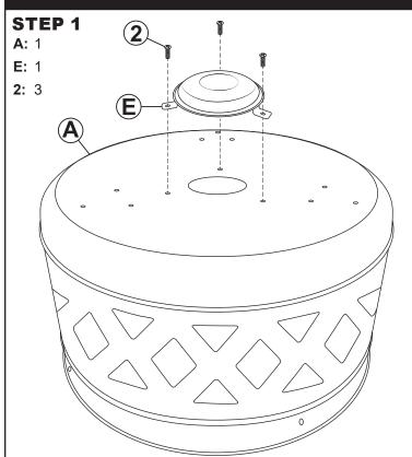
Securely fasten Ash Tray (E) to the bottom of Smokeless Fire-Bowl (A) using three M6x12mm Bolts (2).
