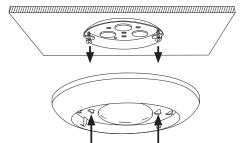
Re-install DSK lens back on by twisting lens clockwise.
