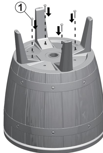
Use one M3.9x19mm Screw (1) to securely fasten each leg to the cooler.
