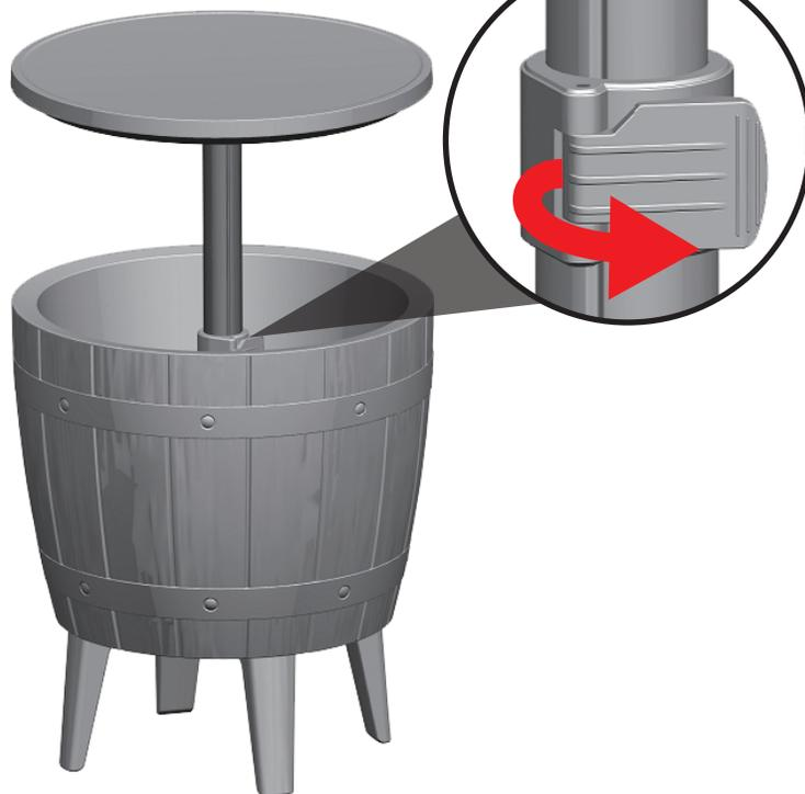
Carefully extend the tabletop/lid to the highest level and lock into position with the lever, as shown.
