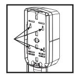
This dispenser is equipped with a universal back plate to allow for easy installation. Before drilling, open dispenser and check existing hardware on wall for alignment.
