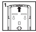
Open dispenser by pushing on cover latch until it releases.
