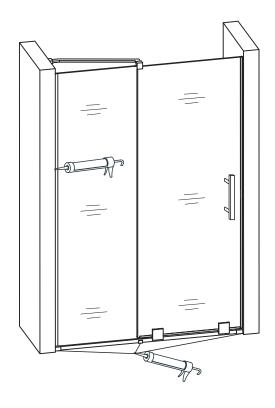
The sealant should be applied to the outside edge.
