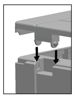
**IMPORTANT:** Use caution when attaching the lid; too much force may cause the resin to crack.
