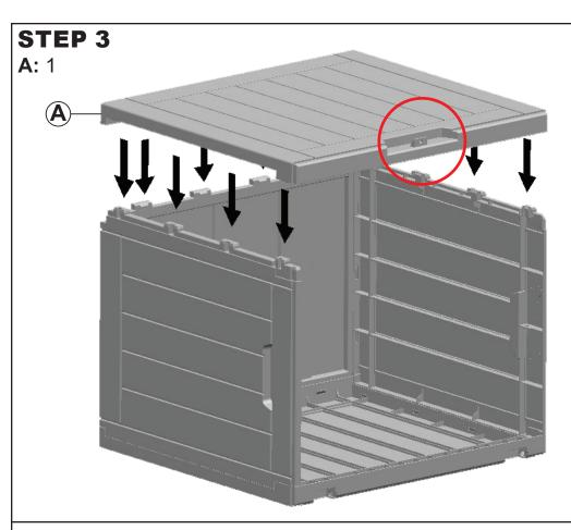
**IMPORTANT:** Ensure the groove on the front panel is installed on the same as the handles in the side panels as indicated in the picture.
