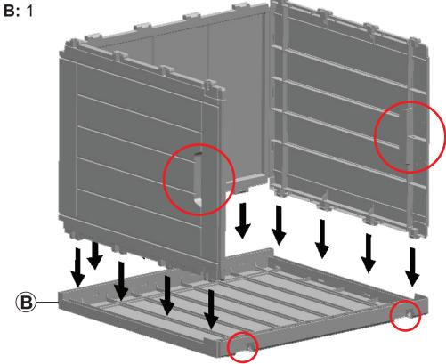
**IMPORTANT:** Ensure the handles in the side panels are installed on the same side as the hinge grooves in the back panel as indicated in the picture.
