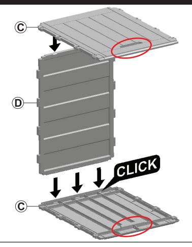
**IMPORTANT:** Ensure the handles in the side panels are installed on the opposite side of the bottom panel.
