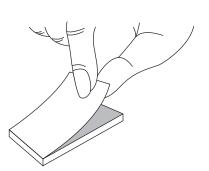
Remove the paper backing from the silicon pads.
