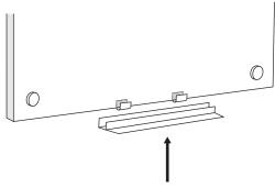
Push the tray onto the silicon pads.
