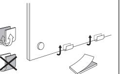
Install the silicon pads onto the bottom of the glass board.
