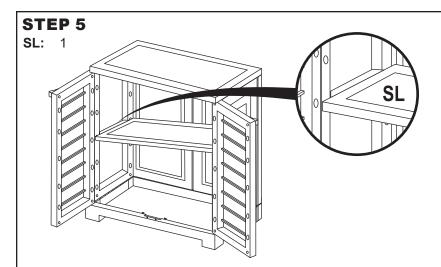
Insert Shelf (SL) into the unit at a slight angle and align the shelf with one side of the unit. Then, gently press on the opposite side of the shelf until the shelf locks into place.
