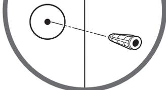
**Note:** If mounting into plaster or drywall, follow this step and use the wall anchors provided.
