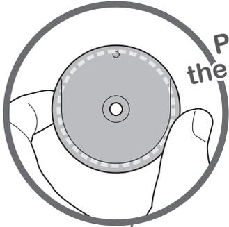
Mark drill holes with a pencil through the center of each wall cup.
