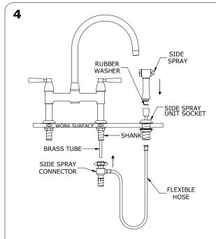
Please note: If there is a low flow at the hand spray, reinstall the side spray connector: Remove the hose and
