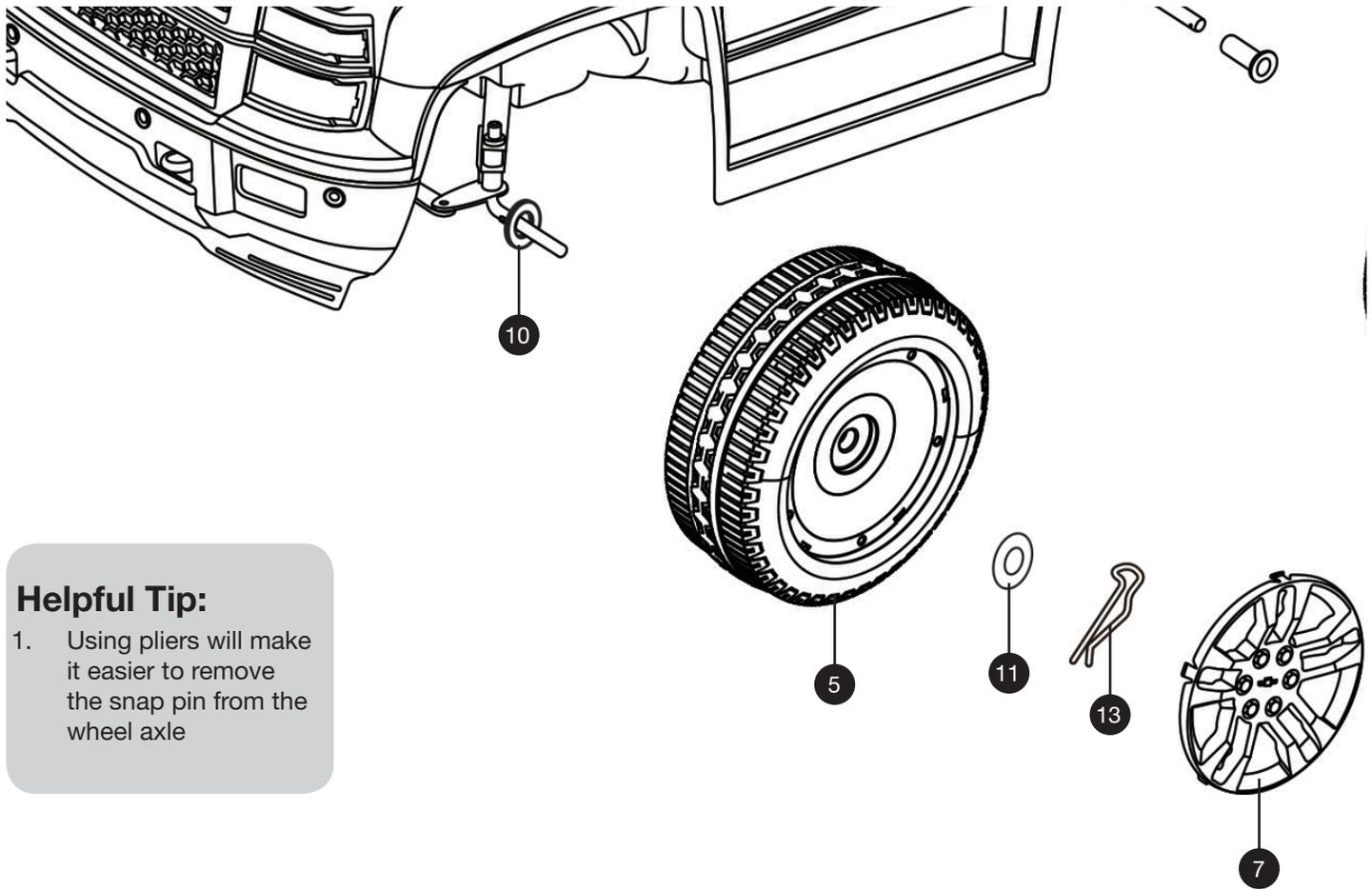
1. Locate the  $\phi 10$  Thick Washers (10), the  $\phi 10$  thin washers (11), and snap pins (13) from blister pack.
