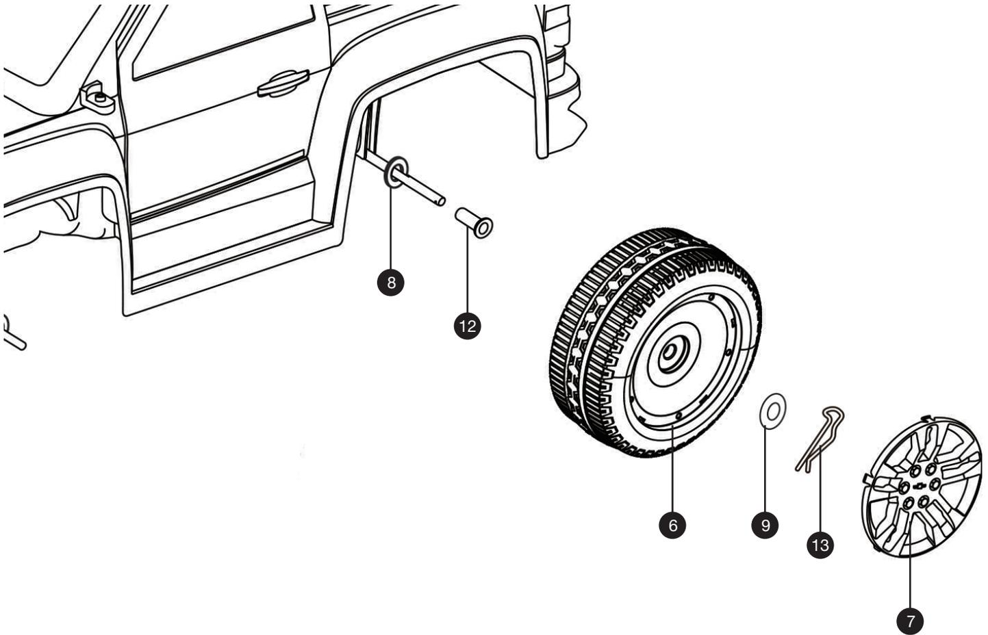
1. Locate the rear  $\Phi 12$  thick washer (8), the thin washer (9), the snap pin (13), and inner wheel spacer (12) from blister pack.
