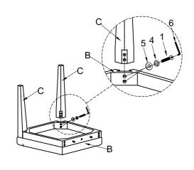
DO NOT TIGHTEN BOLTS COMPLETELY
