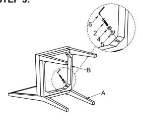
DO NOT TIGHTEN BOLTS COMPLETELY
