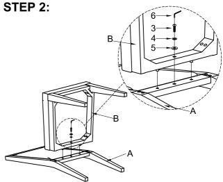
DO NOT TIGHTEN BOLTS COMPLETELY
