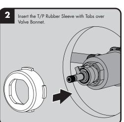
Be sure to have properly adjusted the Temperature Limiting Stop (TLS) as per the Valve Installation Instructions before installing Valve Trim. Slide Trim Sleeve over the Rubber Sleeve. Ensure the tabs are properly seated within the grooves of the Trim Sleeve  $\mathbb{O}$
