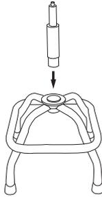
2. Carefully position the Seat assembly over the center rod in the Pneumatic Cylinder and press down.
