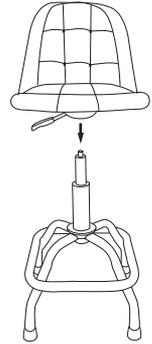
3. Firmly press down on the seat to ensure all three pieces have properly seated and fit together tightly. You should now be able to lift the seat up by the cushion without it coming off of the Pneumatic Cylinder. If the seat comes off, repeat steps 2 and 3.
