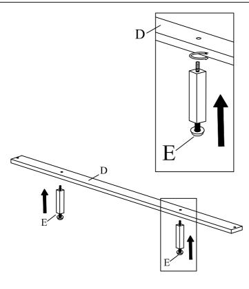
STEP 3: ATTACH THE SUPPORT LEGS (E) TO THE SUPPORT SLAT (D).
