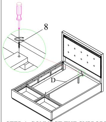
STEP 4: CONNECT THE SUPPORT SLAT ASSEMBLY TO THE HEADBOARD AND FOOTBOARD SUPPORT SLAT CLEAT USING TWO WOOD SCREWS (8).
