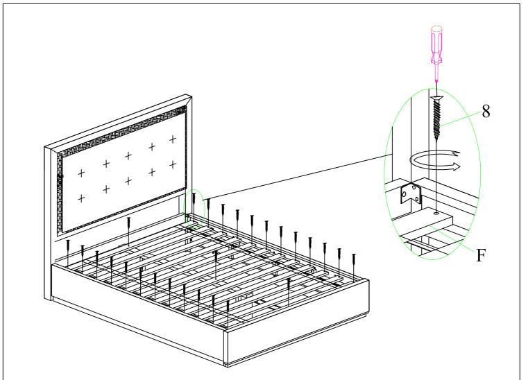
STEP 5: FOLLOWING THE ILLUSTRATION, PLACE AND CONNECT THE SLAT ROLL (F) TO THE BED WITH THE PROVIDED WOOD SCREWS.
