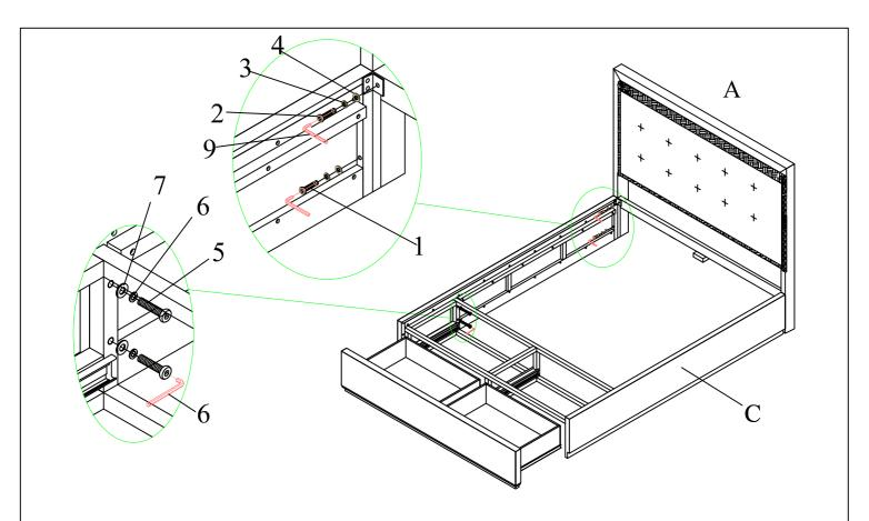
STEP 2: REPEAT STEP ONE FOR THE SECOND SIDE RAIL. TIGHTEN ALL ALLEN BOLTS FROM STEP 1 AND 2 COMPLETELY WITH THE ALLEN KEY (9).
