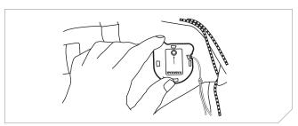
9. Press down on the inflator and turn the locking ring clockwise until it is locked in place.
