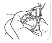
Secure the conversion cap to the hydrostatic water inlet by applying pressure to the cap at the metal clip until it locks in place.
