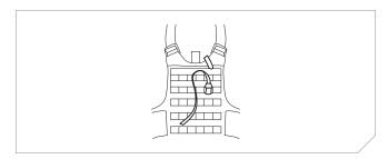
4. Remove male buckle from webbing strap attached to the Ratis™ LPU body.
