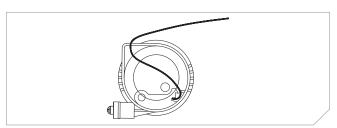
When the Hammar Automatic Inflator is submerged under more than approximately four inches of water, the hydrostatic inlet valve opens, allowing water contact with the water-sensitive element. The element releases a stainless steel coil spring, driving a needle into the end of the gas cylinder, puncturing it and allowing the gas to fill the Ratis™ LPU. The Ratis™ LPU should fully inflate within five seconds.
