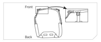
3. Feed the buckle all the way through the harness slot.
