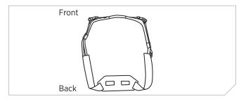
2. Loop one of the male buckle straps of the front lobe through the front harness slot.
