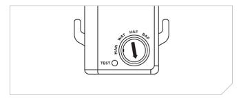
Turn the Mode Selector to the desired position, based on the inflatable requirements. See Hammar Electronic Inflator Manual for more information.
