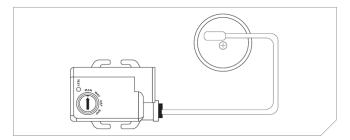
The Hammar Electronic Inflator is a battery-powered electronic inflator that can activate at various water depths or submersion times defined by a selector switch. A manual pull handle can also activate the inflator. The inflator electronics are connected to a gas cylinder by a cable. When the inflation conditions defined by the selector switch are met, the inflator sends an electrical signal through the cable to ignite an explosive charge at the cylinder to release the gas.
