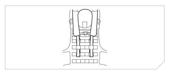
9. **IMPORTANT!** Close the sternum strap in front of the inflatable. This holds the bladder lobes together in the inflated condition. If it is not fastened, self-righting performance will be negatively affected.
