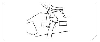
12. Pull the strap tight so the Ratis™ LPU is securely attached in place.
