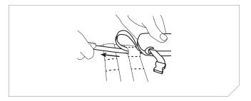
5. Pull the strap tight so the inflatable is securely attached in place. The tighter this connection, the better the performance. Any slack in this connection allows the inflatable chamber to separate from the body/armor carrier in the inflated condition.
