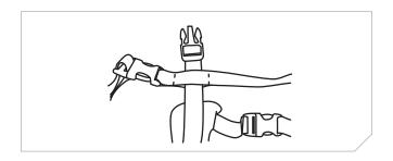
4. Clip the male buckle to the female buckle under the inflatable lobe.
