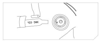
8. Place the new inflator on top of the cylinder assembly.
