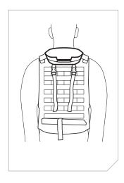
NOTE: EXACT ATTACHMENT LOCATIONS WILL VARY BETWEEN DIFFERENT ARMOR CARRIERS AND KIT SET-UP. IN ALL CASES, THE ARMOR CARRIER MUST BE ATTACHED SNUGLY TO THE USER. IF THE CARRIER IS LOOSE, THE RATIS™ LPU MAY RIDE UP AND OVER THE HEAD OF THE USER WHEN INFLATED.
