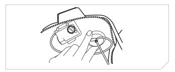
4. Remove the cap from the cylinder assembly.
