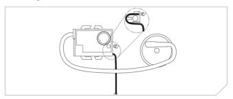
7. Carefully insert the new cylinder assembly into the bladder.
