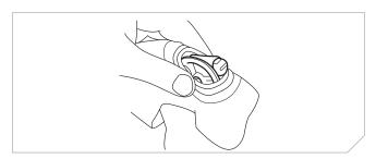
6. Ensure the black pull handle cord tab is inserted in the inflator. If it is not, route the tab underneath the green cable, then route the pull handle cord around the perimeter groove in the plastic tab and insert back into the electronic inflator. The tab should click into place. Significant resistance indicates that the cord is not routed correctly
