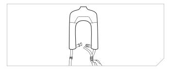
5. Feed the male buckle onto the girth hitch webbing as shown.
