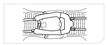
2. Check fit. The Ratis™ LPU should be snug against the armor carrier with webbing straps tightened. The seam joining the lobe fabric panel and the back fabric panel should be approximately in-line with the back of the neck. If the Ratis™ LPU is set too far back on the body, the neck hole will not properly fit in the inflated condition.
