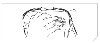
Confirm the indicators on the new cylinder assembly and inflator are green and carefully insert the new cylinder assembly into the bladder.
