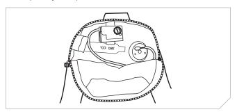
3. While holding the cylinder through the bladder, unscrew the Hammar inflator cap from the cylinder assembly.
