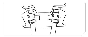
14. Inspect and confirm that all Ratis™ LPU straps are tightly attached to the harness and that no webbing or attachments are twisted. The harness should sit flat against the back. The collar of the Ratis™ LPU should be close to the neckline of the user for optimal performance.
