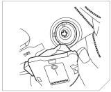
5. Pinch to fold the sealing ring, to allow the removal of the cylinder assembly. Visually check the sealing ring for any damage.
