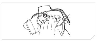
10. While holding the cylinder through the bladder, screw the Hammar inflator cap to the cylinder assembly to close the circuit.
