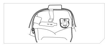
3. While holding the cylinder through the bladder, use the Hammar Key and insert it between the yellow inflator cap and the black locking ring. Turn the key counter clockwise, which will cause the black portion of the cap to rotate counter-clockwise.
