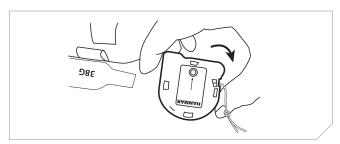
10. Fold the pull handle of the new inflator in half, pass it through the buttonhole of the left lobe, and attach it to the Velcro patch.
