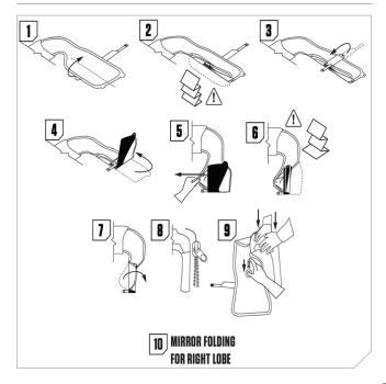
7. Starting with the wearer's left lobe, fold the inside of the bladder lobe towards the outside. Pull taut so the fold edge is over top of the inside edge of the front attachment buckle.
