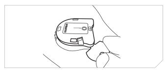
Keep turning the locking ring counter-clockwise and remove the cap from the cylinder assembly. The used inflator cap can be scrapped.
