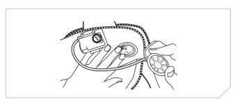
5. Pinch to fold the sealing ring to allow the removal of the cylinder assembly. Visually check the sealing ring for any damage.
