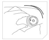
Align the cylinder with the location image on the bladder and make sure the sealing ring rests on the cylinder assembly and does not capture extra folds of the bladder film.
