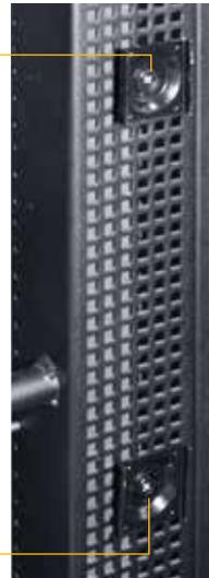
Simply attach mounting clips in desired location for an easy installation. Snap the VT-EXT into clips for a sturdy and secure fit and plug into a Panamax/Furman power conditioner. The plastic spacers in clips provide ground isolation from the rack.
