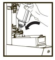
**3.** Push refill pump down into pump house, ensuring collar snaps into place.
