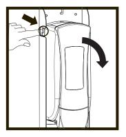
**2.** Open dispenser by pushing on one of the dual side latches until it releases and pull down on front cover.
