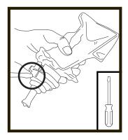
**6.** Use flat head screwdriver to remove collar and cap on refill bottle and discard.
