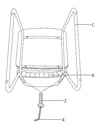
Use Flat Head Bolt (2) to assemble the Back (A) on the Base (C). Use Allen Key (4) to tighten.
