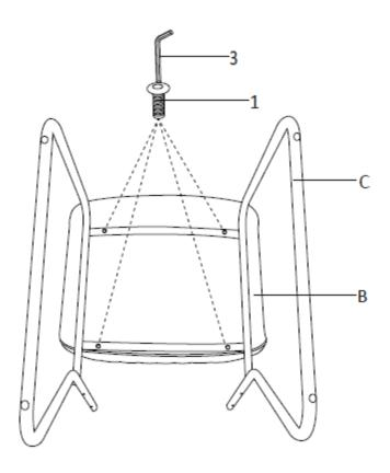
Place the Seat (B) on the Base (C) with Round Head Bolt (1). Use Allen Key (3) to tighten.
